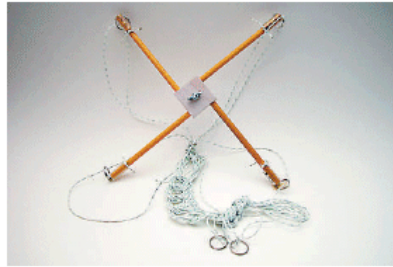
An image of the completed Picavet with its suspension lines daisy chained.
