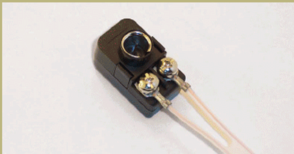
Matching transformer connected to FM antenna.
