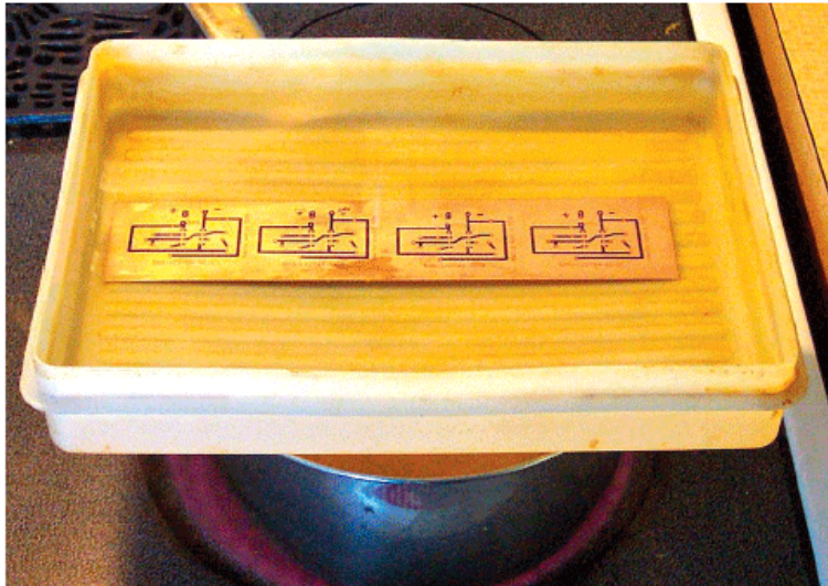
Etch the PCB on the stove.
