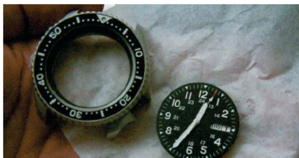
This 7S26 sports a new dial, crystal, and hands. Case and bracelet were bead-blasted.
