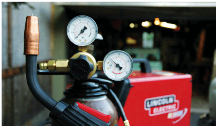
The prettiest “tube-of-toothpaste” welds are accomplished by using shielding gas.
