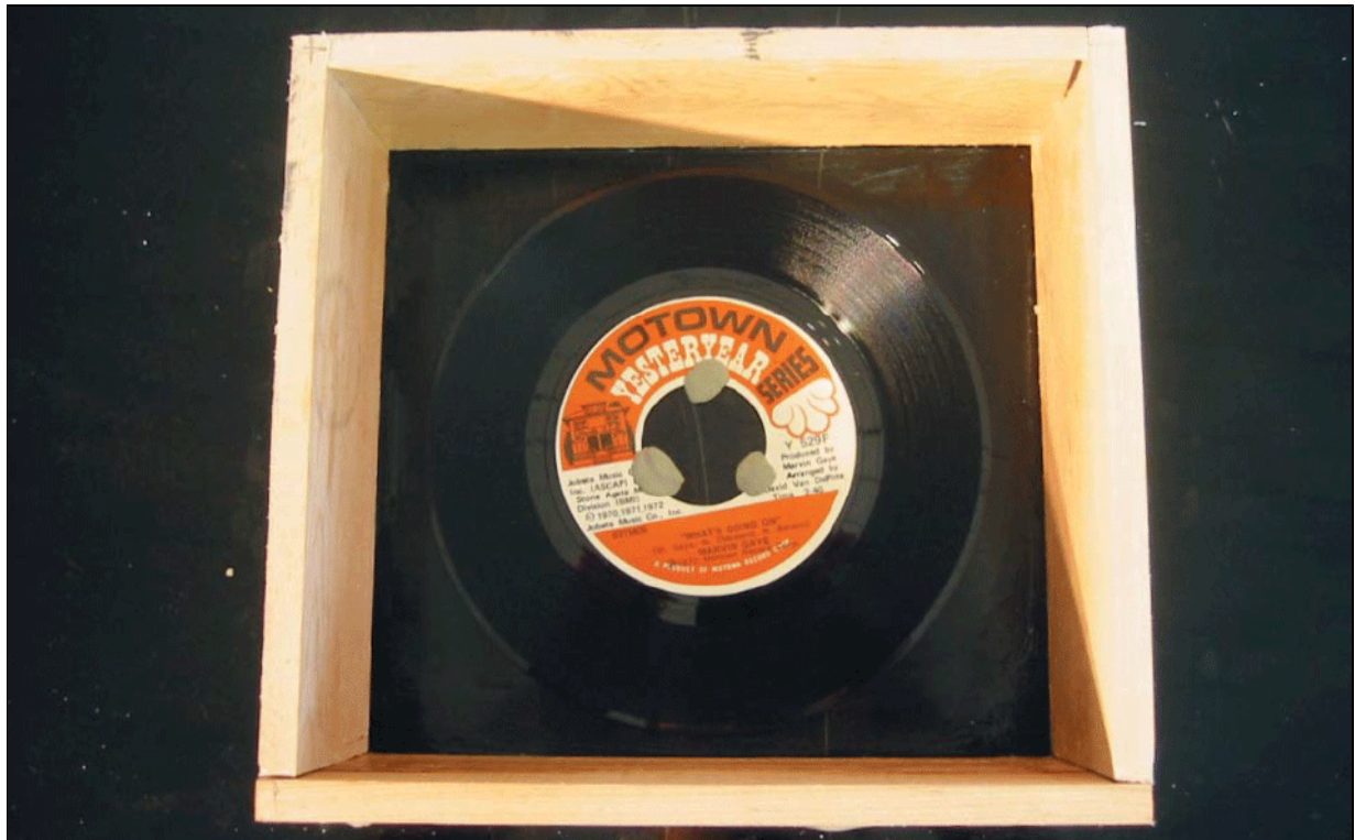
Fig. 1: Place the record you want to duplicate in a box that has been taped up along the corner edges to prevent leakage. You'll then pour enough liquid silicone into
