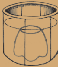
Make base mold from silicone
