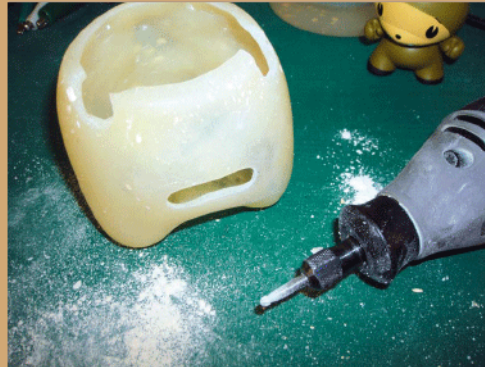
After the resin cures, you can use a Dremel tool to machine the base.
