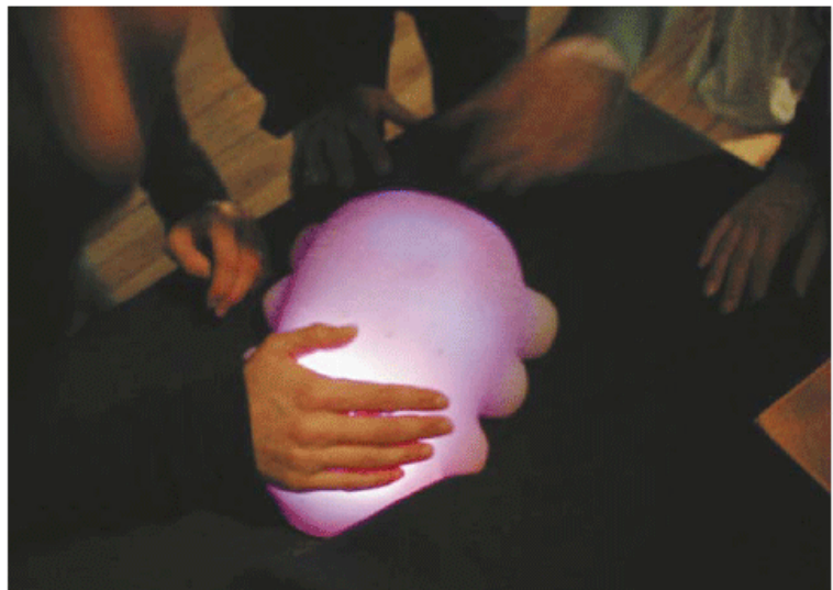
The Platypus Amoeba has touch sensors on its back, and responds to petting with lights and sounds.
