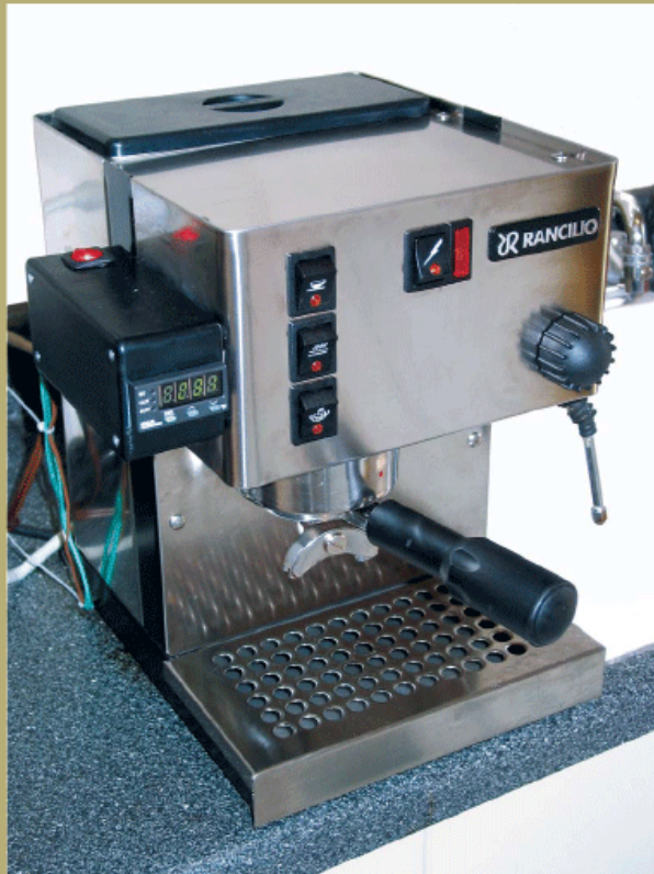
The Rancilio Silvia outfitted with temperature control.
