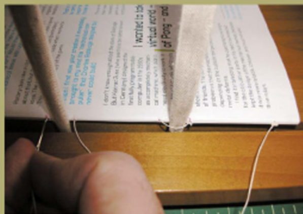
Use a heavy needle to penetrate the paper. The three tapes (one is shown here) run behind the signatures.
