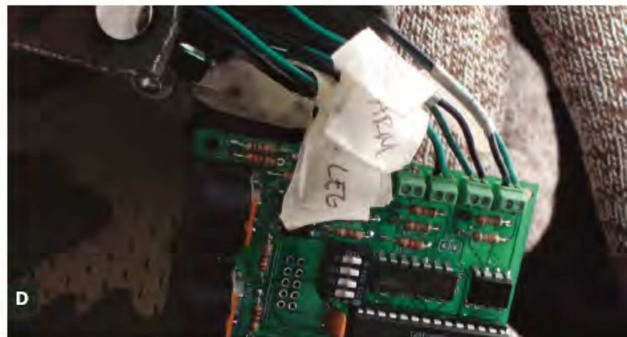
Fig. C: Partially assembled sock monkey, with sensor wires and reinforcement sewn at base of monkey's back. Fig. D: Sensor wires connected to MIDIsense board.
