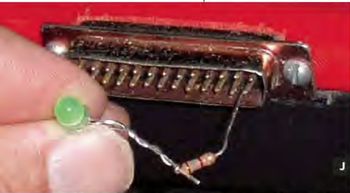
Fig. H: The matrix tester is made from an LED and a 1k resistor. Fig. I: Use this circuit to determine the polarity of the phototransistor. Fig. J: Attach the resistor to the ground pin and touch the LED anode to each pin,
