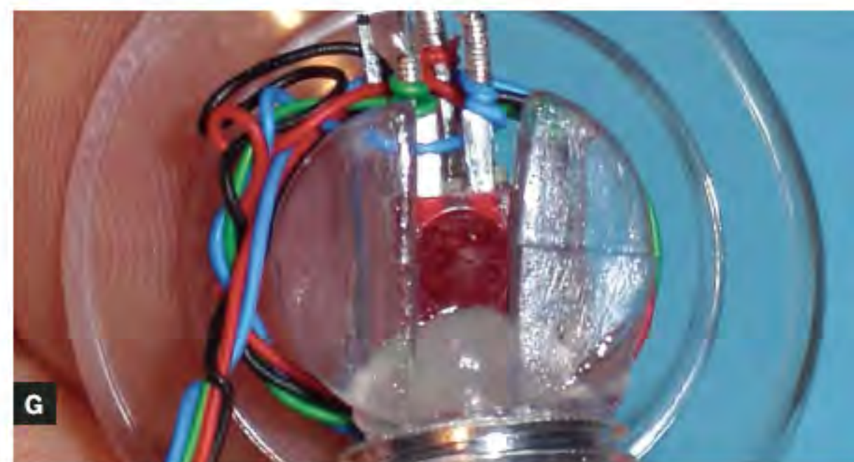
together with tape and insert into suction cup. Fig. G: Apply silicone glue to the assembly.
