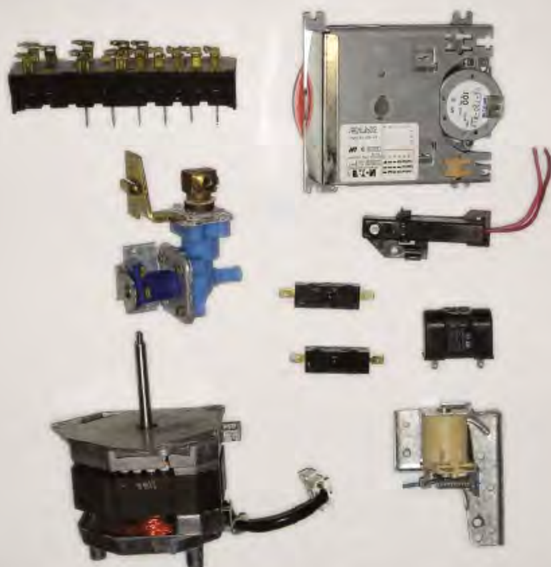
Fig. A: A few minutes' work with common hand tools and a generous application of maker philosophy yields motors, switches, valves, and solenoids, all taken from my curbside find. Fig. B: The "brains" of the dishwasher,
