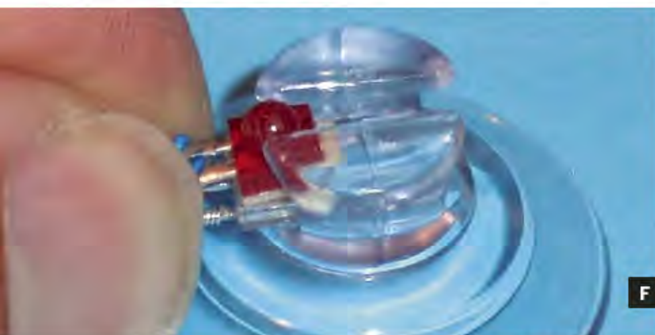
Assembling a suction cup sensor. Fig. D: Each suction cup sensor consists of an LED and a phototransistor. Fig. E: Use a wire wrap tool to attach connector wires to component leads. Fig. F: Stick LED and phototransistor
