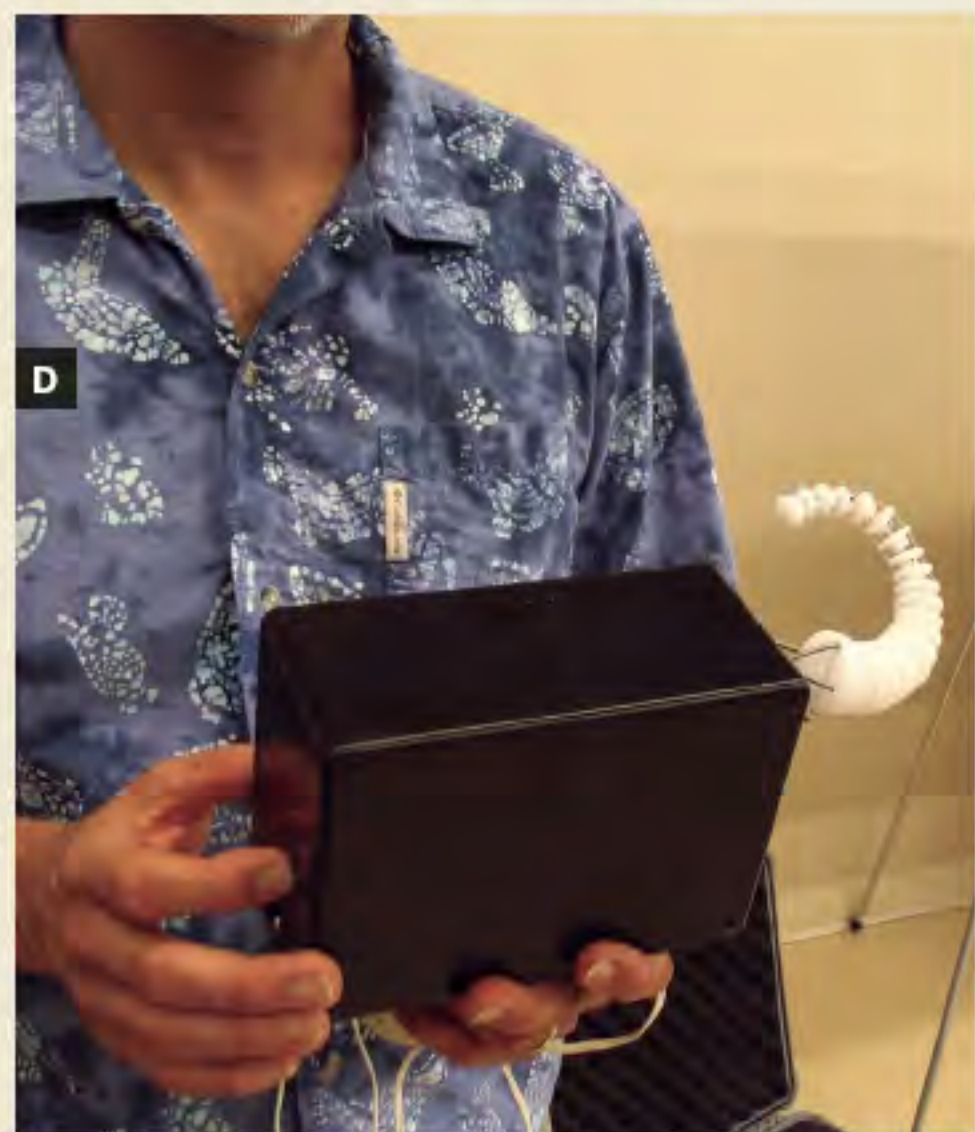
A. The Anatomy of the Furby by artist Kelly Heaton, who once made an interactive Furby wall. B. A UgoBee engineer troubleshoots a locomotion problem with Pleo. C. Caleb Chung's lab is an unassuming box in a small office park outside of Boise. D. A Pleo tail-testing unit. E. Pleo in a classic pose.
