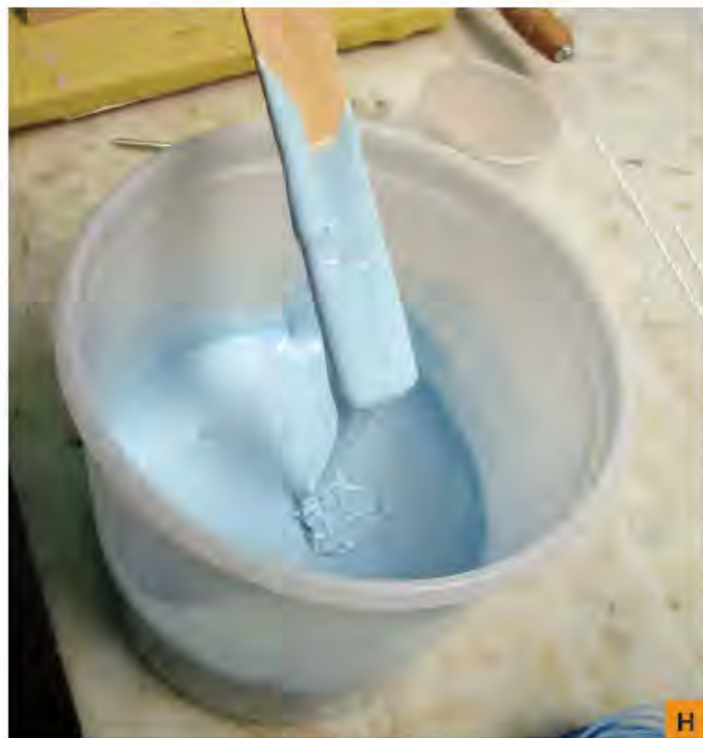
Fig. G: The silicone before mixing. Fig H: The silicone after mixing. If you see any white streaks, you're not nearly done. Fig I: Pouring the silicone. You should pour thinner than this, unless you have an evacuator to put the mold into immediately afterwards (like I did).
