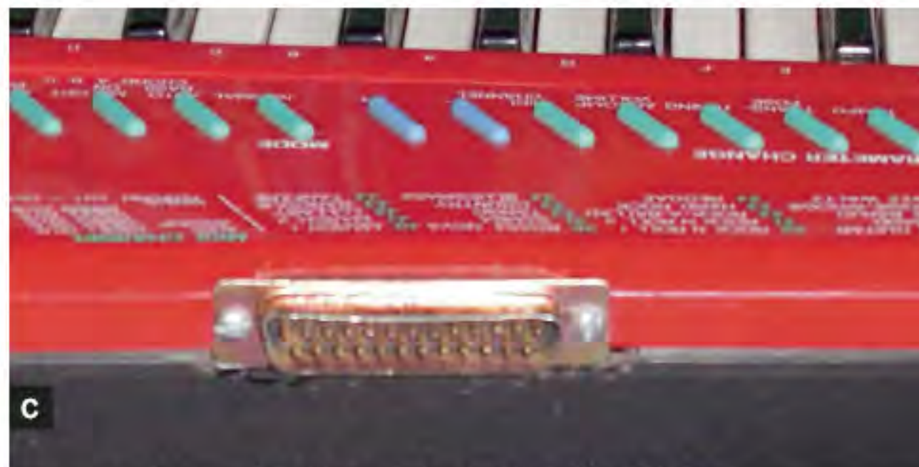
power and ground. Solder each wire from the D25 connector to the circuit-board pins on top of the keyboard cable. Fig. C: Check the connections, close the case, and attach the D25 connector to the back of the keyboard.
