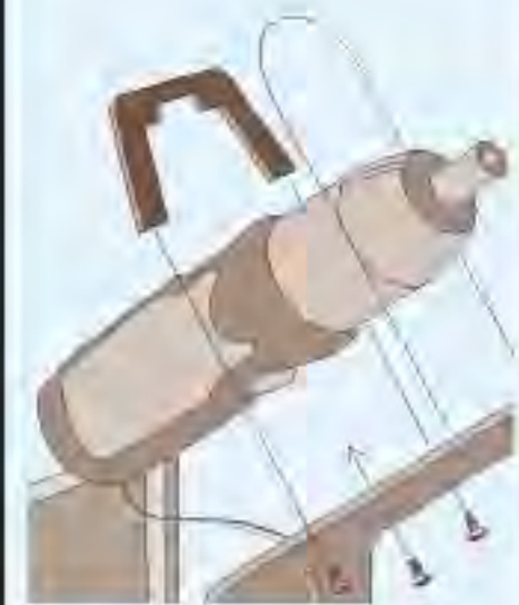
Plastic hold-down and wire loop secure the screwdriver while another screw keeps its On button pushed in.
