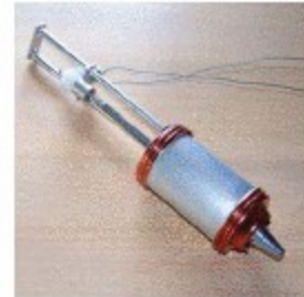
CLOCKWISE FROM LEFT: The Fab@Home extruder is a syringe driven by a linear actuator; the Stratasys Dimension 3D printer extrudes a filament of heated plastic; the author's DIY cookie press, retrofitted for computer control with a $6 motor.
