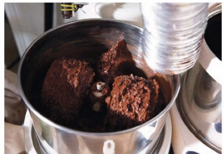
RIGHT: These wet mixers, now used as chocolate melangers, were made to mix Indian curries. Temperature control is essential when making chocolate, so Heckert took Childs' design and outfitted the mixers with infrared sensors and cheap space heaters that blow just the right amount of hot air on the oozing goodness.
