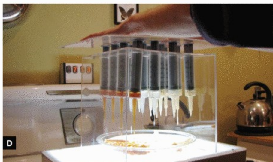
amounts of chemicals, so a high-quality scale is a must. Fig. D: Squirt drops into the setting bath, controlling the size of the drops by the pressure you put on the plunger. Make the drops about the size of salmon eggs.
