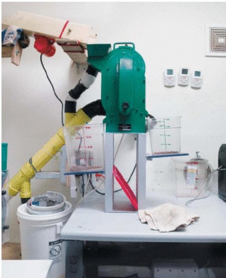
TOP LEFT: A converted and customized coffee bean roaster works like a champ for cacao. TOP RIGHT: The Crankenstein is a grinder for beer hops, customized with a wider gap between the rollers for cocoa beans to fit through. BOTTOM LEFT: After it's ground, winnowers are used to blow off the bean's shell from the meat. Childs modified plans he found online for a winnower designed for agricultural use in developing nations. They cobbled together a spare blower from Heckert's shop using a Shop-Vac found on a sidewalk, and made a vibrating feeder using a vibrator from another old machine. After adding some PVC pipe, the total cost was $12.
