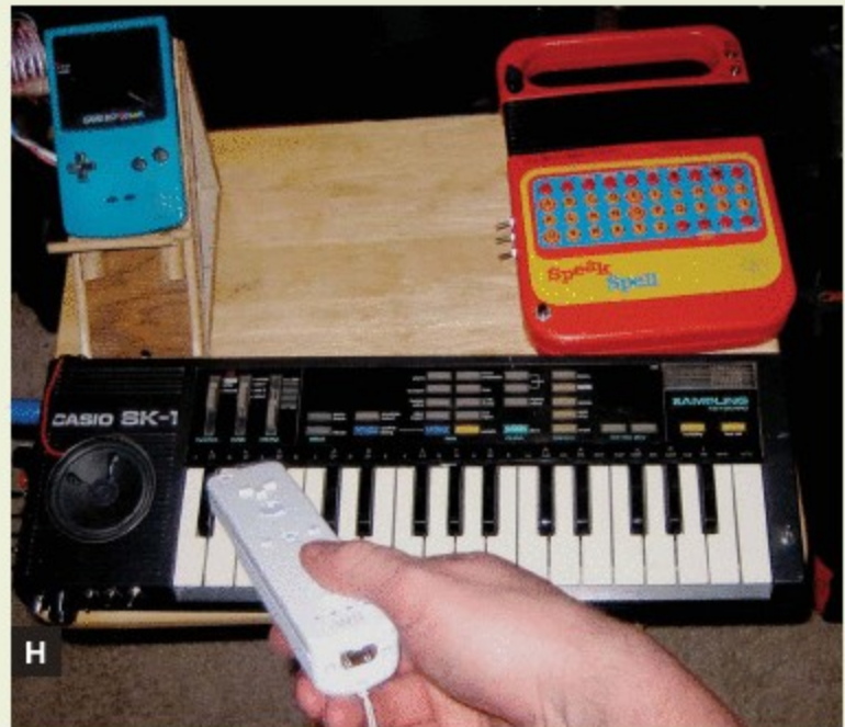
Fig. H: Wiimote-controlling a Casio SK-1 keyboard and a Speak & Spell toy.
