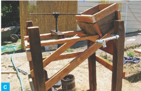
Fig. A: The chicken run. We started out with 4 and grew the flock to 15 because the chickens were such good calorie producers. Fig. B: Cold frames with new starts. Fig. C: A modified apple press with a macerator that the Energy Garden team designed. Fig. D: The moonshine still distilling apple cider into ethanol fuel.
