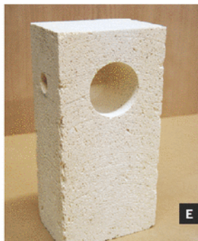
Fig. A: Mark the chamber location on the firebrick. Fig. B: Drill the firebrick slowly. Fig. C: Position the flame hole so that flame will circulate around the chamber. Fig. D: Drill the flame hole.
