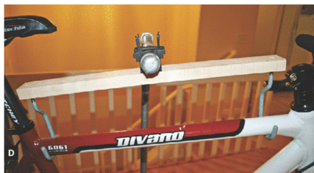
upright with hose clamps. Fig. D: Pipe hangers connect the horizontal pipe to the wooden board. Utility hooks screwed into the board hang down to hold the bicycle.
