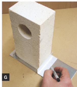
Fig. E: Flame hole and chamber drilled. Fig. F: Drill the vent hole in back. Fig. G: To build the frame, first mark the edge of the aluminum angle on the plate.
