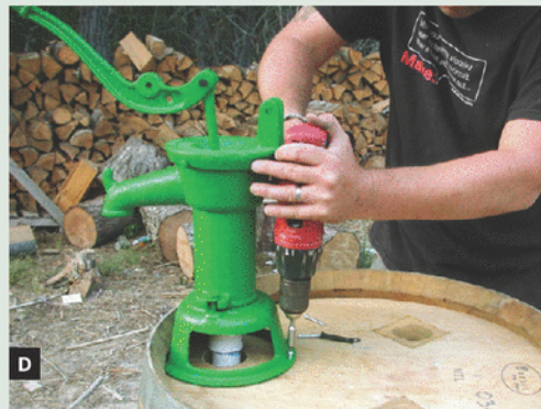
Fig. C: Measure the down tube to extend from the adapter under the pump valve to the barrel's bottom. Fig. D: Wear proper attire while screwing the pump onto the barrel top; a MAKE shirt always works!
