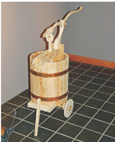
CLEAN ENERGY: Laundry machine prototype in Nepal (top), and a small, cartable version of the machine built as a woodworking project (bottom).
