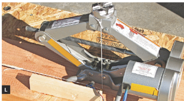
Fig. L: Center the trim pots, center the jack and the pot, then tension the string.
