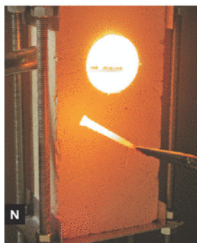
supported and secured by nuts on threaded rods. Fig. L: Firebrick in place between the top and bottom plates. Fig. M: Grate made from cut nails tapped down into the brick. Fig. N: Micro forge in operation.
