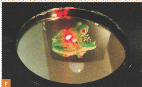
Fig. F: Aiming a laser pointer beam at the image of a frog causes a small spot on the image to be illuminated. Fig. G: Typical ray paths from object to image and beyond. Fig. H: Two concave mirrors can be used to demonstrate images formed by reflection — with light, heat, or sound. Here, sound from a ticking watch is focused onto a flame, causing it to flicker. Light from the flame forms an image on the watch.
