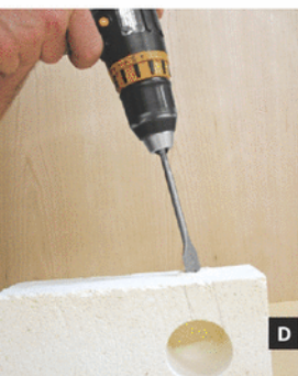
Fig. A: Mark the chamber location on the firebrick. Fig. B: Drill the firebrick slowly. Fig. C: Position the flame hole so that flame will circulate around the chamber. Fig. D: Drill the flame hole.
