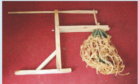
FOUR-DOLLAR WASHING MACHINE: Nepalese villagers test a prototype of the off-grid laundry machine, manufactured locally for $4 using wood, jute rope, and bamboo tubes.
